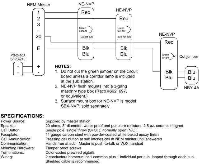
Use Aiphone #822202 or #821802 for homerun wiring, #822206 for up to 5 stations<br/>on each run, or #822210 for up to 9 stations on each run.Wiring Distance:420' with 22AWG; 1,000' with 18AWG.
